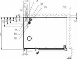
GΑ Gas connection EΑ Electrical connection STL Control line LOA Performance optimization system PΑ Equipotential bonding ΚE Network interface Cold water ΚW EW Soft water Drain water Α ΑL Exhaust air
